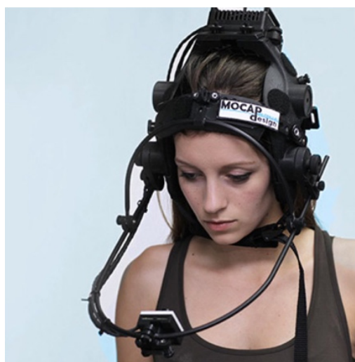
Figure 8. showcases the facial motion capture system, complete with the helmet. [19]
